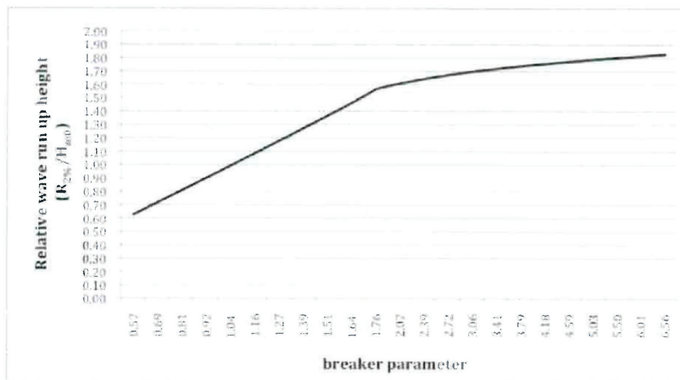
Figure 4-11 Wave run-up curve for rocky shoreline at Port Elizabeth ( \lambda f = 0.45 )
