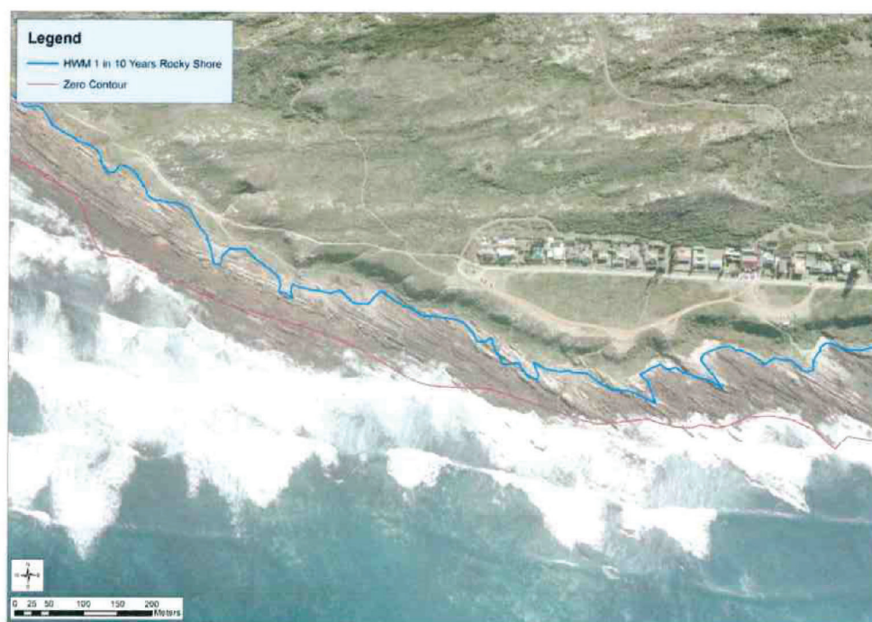
Figure 4-12: HWM modelling using Eurotop manual for rocky coastline at Schoenmakerskop , west of Cape Recife
