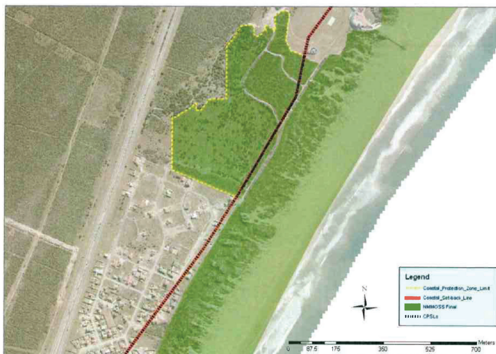
Figure 4-21: CSL and CPZL for Blue Water Bay to Wells Estate inside of Algoa Bay.
