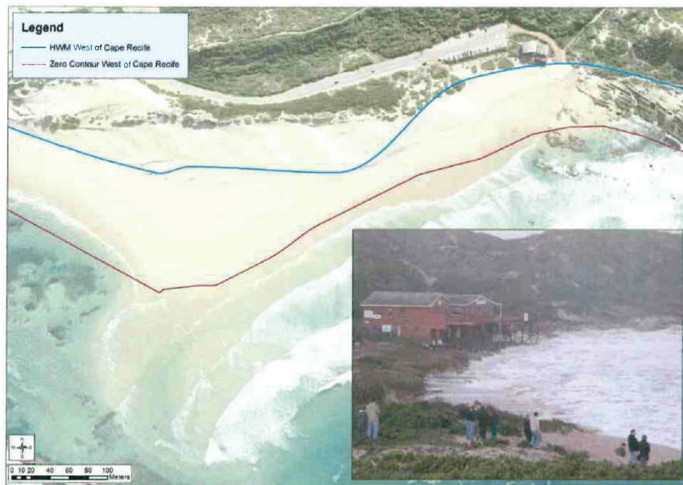
Figure 4-9: Modelled HWM at Sardinia Bay west of Cape Recife, the results are verified by the insert in the lower right hand corner showing extreme wave run up during the September 2008 storm event, note the position of run up in relation to the two structures.
