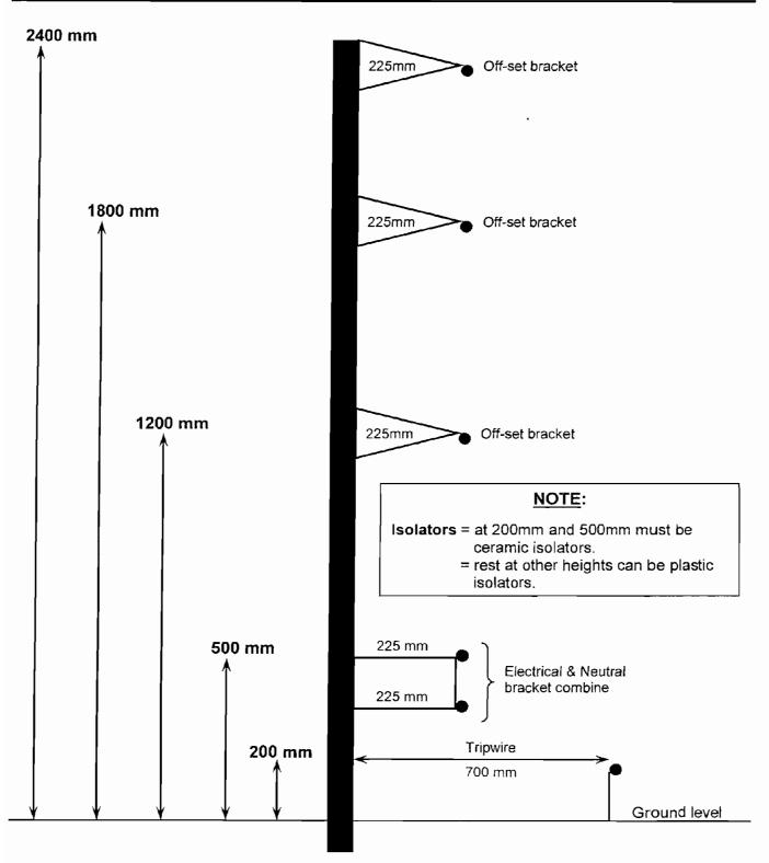
FIGURE 4: ELECTRICAL WIRE SPECIFICATIONS FOR FENCE TYPE 4
