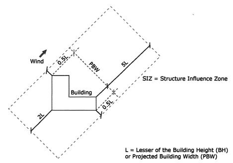
Figure 3. Structure influence zone for downwash analyses
