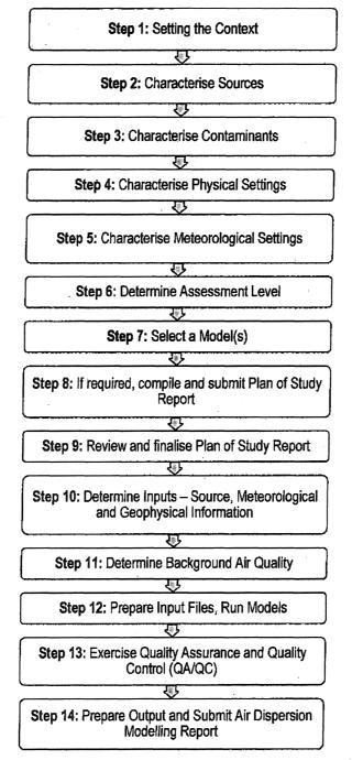
Figure 1. The 14 Steps to Good Modelling Practice (adapted from British Columbia 2008).
