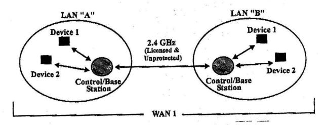
According to European Telecommunications Standards (ETS), a Local Area Network or LAN is defined as "a group of user stations each of which can communicate with at least one other using a common transmission medium commonly managed".
