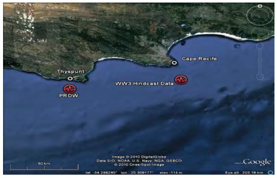
Figure A-10: Wave data extraction locations for Step 1 and Step 2, PRDW refraction modelling extraction in approximately 30m water depth offshore Thyspunt and WW3 hindcast data extracted for a position directly offshore of Cape Recife respectively.
