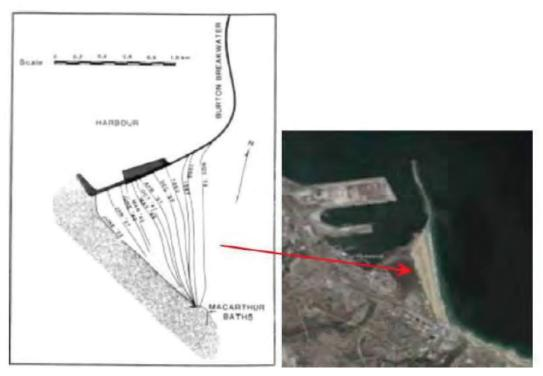
Figure A-9: Left: Accretion of sand at King's Beach. From Lord et al, (1985). Right: Current aerial photo of King's Beach - the beach is now "over-flowing\_ and moving around the breakwater and into the approach channel, which requires regular dredging. It is estimated that approximately 1 million cubic meters of beach sand is located off the breakwater.
